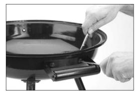
**5.** Attach Handle to Lid with 2 bolts, washers & nuts. **Again, be careful not to overtighten bolts as this could crack the porcelain finish on the Lid.**
